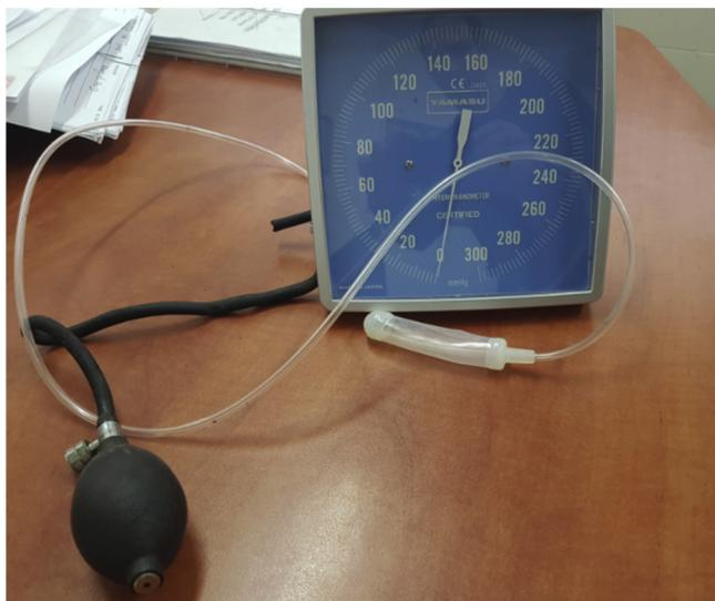
Figure 1. Low-pressure cylindrical algometer. Figure 1 is available in color online at [www.jsm.jsexmed.org](http://www.jsm.jsexmed.org).
